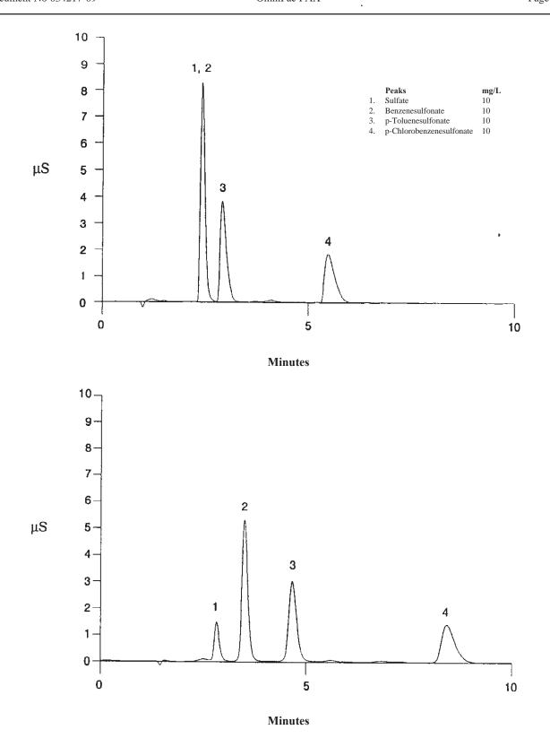
Figure 14 Combined Adsorption and Ion Exchange Retention of One Analyte
