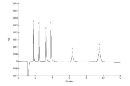
Figure 2 OmniPac PAX-100 Test Chromatogram
