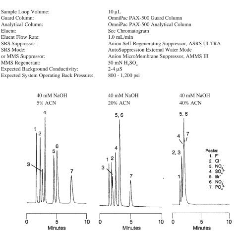
Figure 8 The Effect of Acetonitrile on Times with the Omnipac PAX-500
