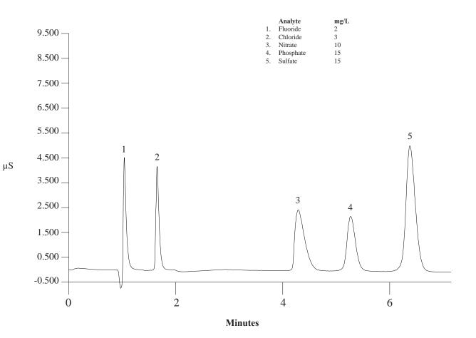
Figure 5 Carbonate Eluent
