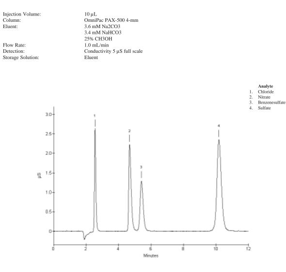
Figure 3 OmniPac PAX-500 Test Chromatogram
