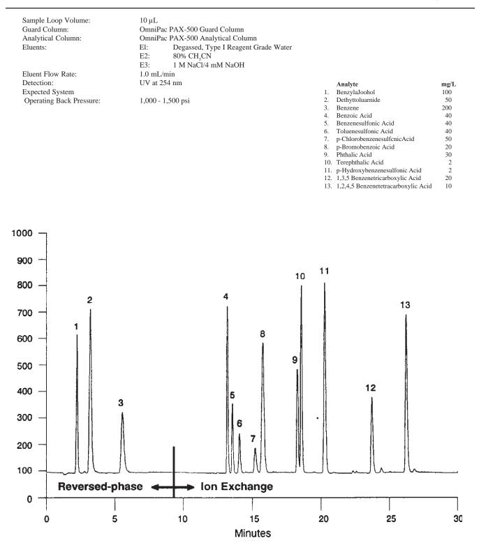
Figure 13 Multi-mode Chromatographic Separation of Ionic and Nonionic Aromatic Compounds
