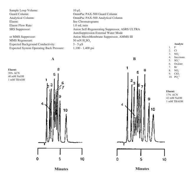
Figure 11 Combined Ion Pair/Ion Exchange Separation on the OmniPac PAX-500
